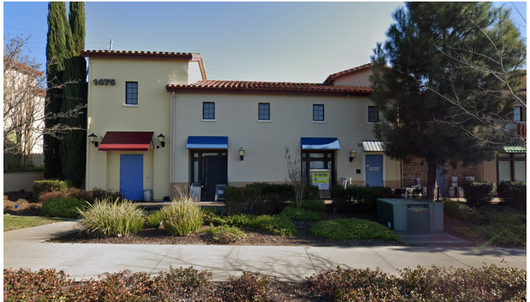
Example of a passive building side designed with faux storefronts, windows, and other features to appear activated.
